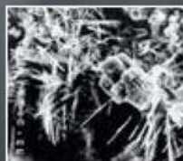
Xypex Crystallization (Initiated)
